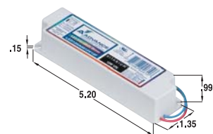
Figure C AC input: 6-inch 18AWG leads Line (black), Neutral (white) DC output: 6-inch 18AWG leads Positive (red), Negative (blue)
