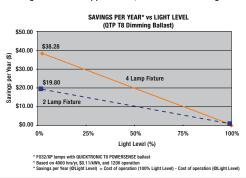
(0-10VDC, Class 1 or 2) are used to control the lighting system. In this daylight harvesting example, each lighting fixture (or fixture row) is controlled by its own photosensor; regulating the light output to compensate for changes in natural daylight. Depending upon the specific application, energy savings of up to 60% compared to fixed output T8 electronic systems can be realized.
