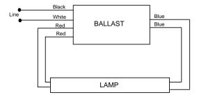
Ballast must be grounded. Install in accordance with National Electric Code.
